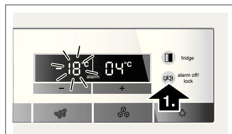
The temperature display indicates for 10 seconds the warmest temperature which was reached in the freezer compartment. Then the set temperature is displayed again.
